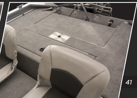
Rear Casting Platform
