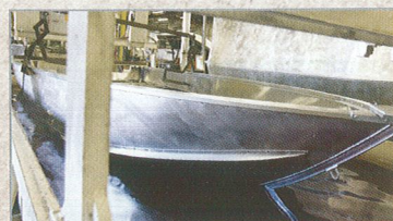
Water-tested hulls ensure rivet and weld integrity
