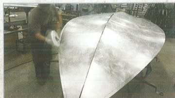
One-piece, single-sheet aluminum finely cut and shaped for the greatest possible inherent shape
