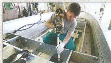
Gas-resistant expansion foam increases buoyancy and quiets the ride
