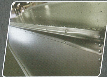
Full-length, oversized spray rails for a drier ride in rough water
