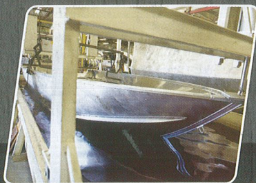
Water tested hulls ensure rivet and weld integrity
