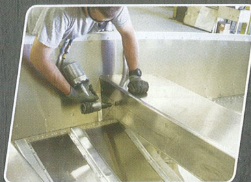
Durable wood-free heavy gauge aluminum seating and stringers
