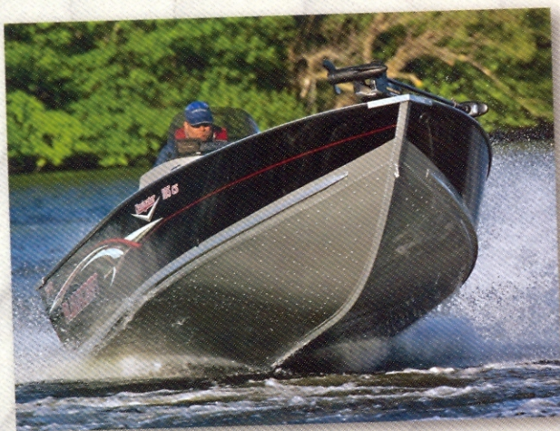
The 2XB Hull (Two X Bottom) is engineered with two aluminum plates riveted together on the hull's bottom. A 2XB Bow is built with twin plates in the bow area.
