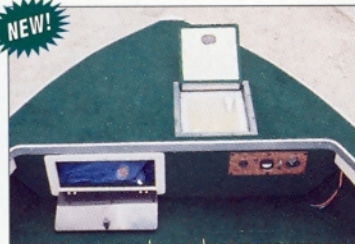
Baitwell/Storage/Battery Condition Gauge
