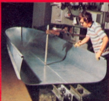
SPOT WELDING SINGLE SEAM OF 2 PRE-FORMED SEMI-V HULL SECTIONS
