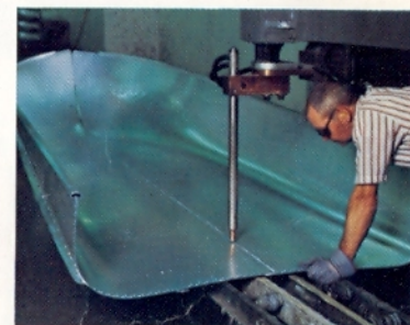
SPOT WELDING SINGLE SEAM OF 2 PREFORMED SEMI-V HULL SECTIONS
