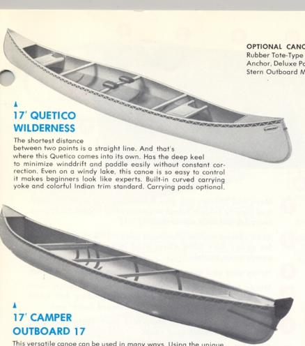
This versatile canoe can be used in many ways. Using the unique wishbone transom which is above the waterline, outboards up to 3.5 hp. can be run. Yet, this 17-footer paddles with the ease of a double end canoe. Painted Dead Grass or Camouflage, it makes an ideal duck boat. CO-17 weighs just 92 pounds. Paint optional.
