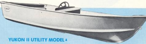
With factory installed mechanical steering and steering deck, the F-9 Lake Master and Yukon II make an ideal utility boat for fishing, water skiing or runabout fun. Utility models F-9 and Yukon II available only with 20" transom. The utility model F-9 is rated for 30 hp. and the Yukon II utility model is rated for 50 hp.
