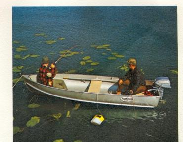
MODEL A FEATURES: Two pair noiseless oarlock sockets . . . Transom drain plug . . . Non-glare, non-skid floor . . . Oar storage brackets . . . Bow eye . . . Flotation, foam . . . Satin finish.
