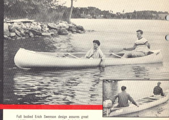
Full bodied Erich Swenson design assures great stability and large carrying capacity. End deck compartments filled with Styrofoam\* provide positive flotation. Constructed for rugged service with strong extruded gunwales. Keel is ½" thick to withstand abrasive action of sand and rock. Read construction details on pages 15, 16 and 17.
